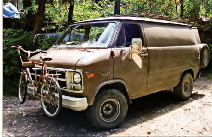
Bruno's '79 GMC van, 4-speed with granny tranny and rear-end positraction on a homebuilt ¾-ton suspension. Motor is 292 long-stroke, single barrel carburetor, manual choke.
