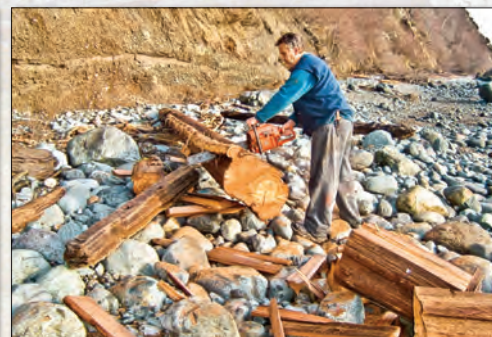
Below: This log washed up on the beach below Bruno's house recently. Here he levers the log up off the rocks, cuts it into two-foot bolts, and then with A-frame and block-and-tackle, hauls them up the cliff, where he split them into shakes. I'm about to bring them down to my place in Northern California, to replace the 35-year-old shakes on my tower.
